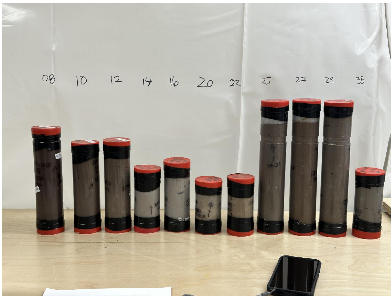
Figure 4. GP17-OCE cores arranged by Station number. The shortest cores (Stations 14-22) occur in the region of the fronts. In almost all cases, the cores showed evidence that there was loss of the bottom portion of the core, possibly at the seafloor.
