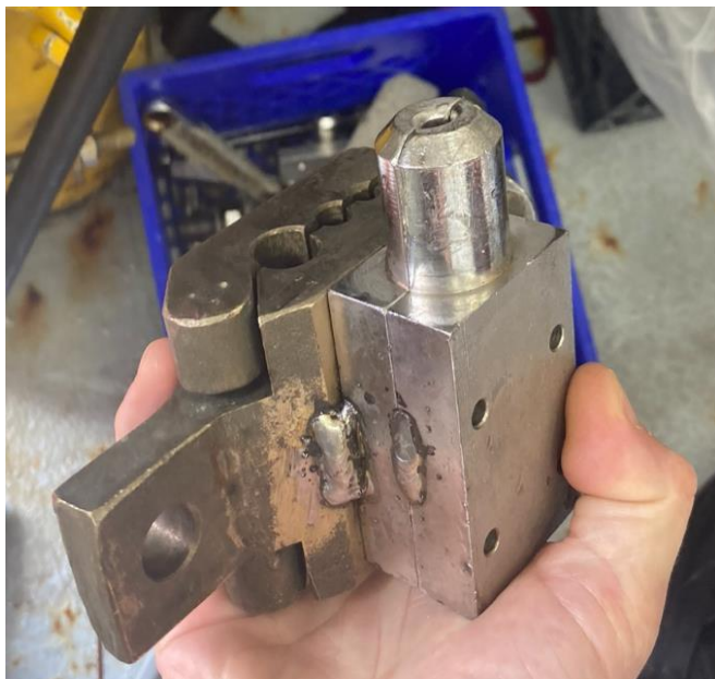
Figure 5. Pump clamp welded by ship's engineers following loss of McLane pumps and associated clamps.
