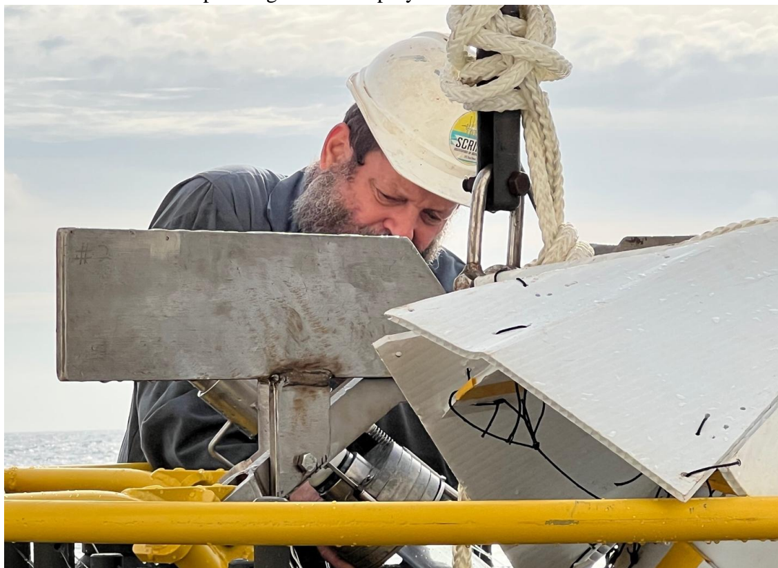
Figure 3. Chief Engineer working to remove the monocrorer after it was deposited on top of Rosette carousel at Station 3, cast 13. Notice the loose wrap of the 5/8" diameter white line around the 0.322" conducting cable.
