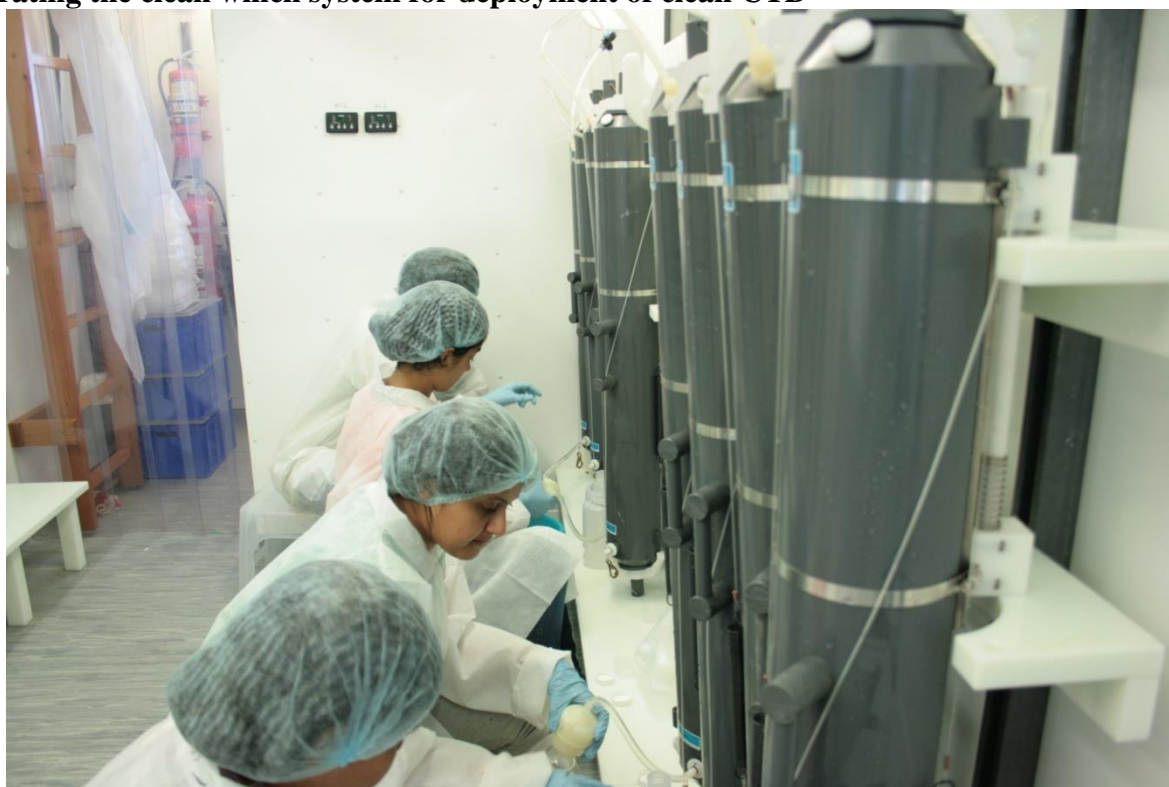
Filtration and sub-sampling of seawater samples inside clean van during cruise SK-304 onboard ORV Sagar Kanya.
