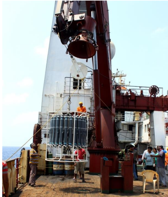
Fig. 3: Clean CTD getting lowered into the sea to obtain Physical Parameters, samples for trace elements, isotopes and Nutrients in the vertical profile of seawater column.
