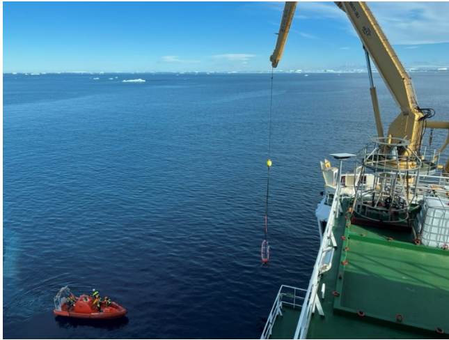
Figure 17-4: Deployment of Caravela from the SDA. The small boat was used to tow the USV away from the ship before release.
