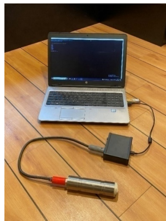
Figure 4.1.4-2: ANB S series pH sensor
