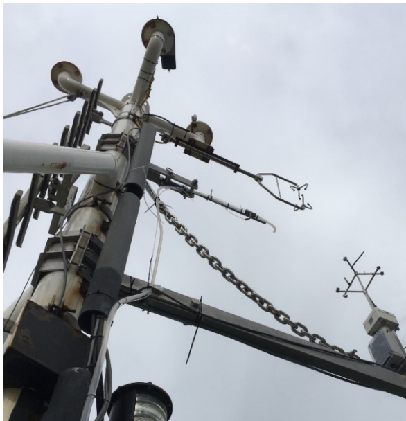
Figure 4.2.1-1: Foremast setup (left photo): The 1/2 in. Teflon gas inlet tube (with 1/8 in. Nitrogen puff tube) is mounted below the ship Metek (top of picture). The LPMS and PML Metek sonic are mounted on a separate horizontal mount at the bottom. Power/data cables (~45 m) and Teflon tubes (~40 m) run from the foremast to the atmospheric lab.
