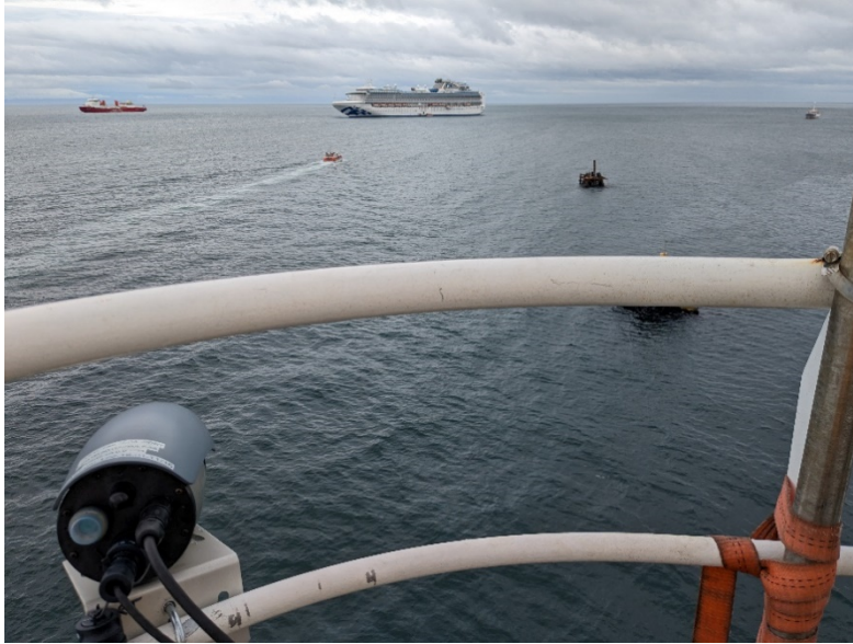
Figure 4.3.1.1-1: Port side CCFC camera setup. The setup was equivalent for the starboard side camera, with camera angle setup to overlap slightly directly forward of the bow.
