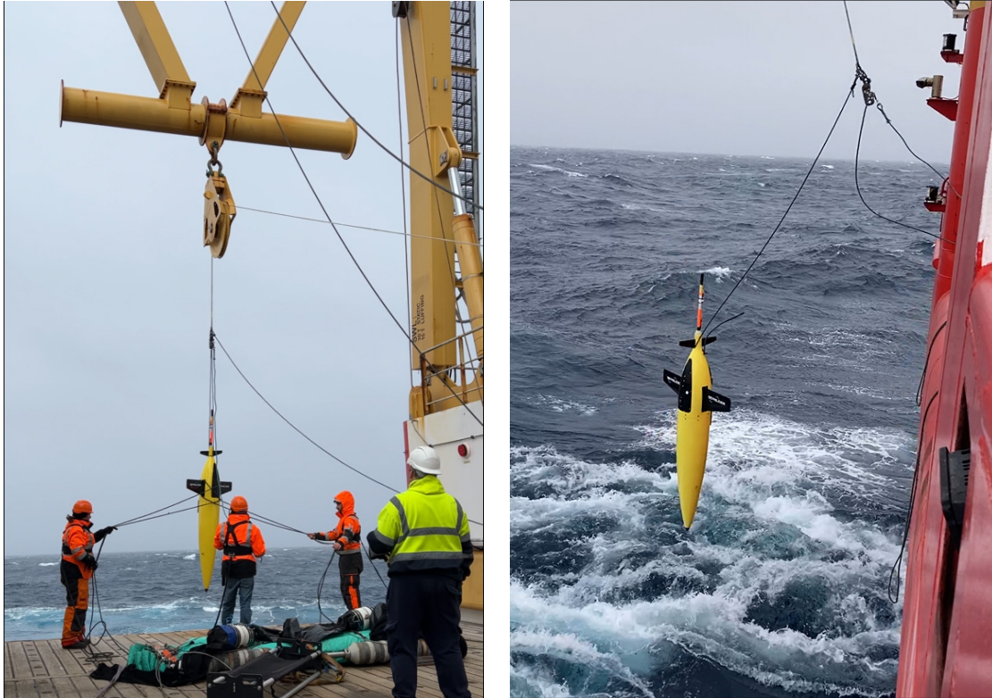
Figure 13.1-11: Deployment of Seaglider using the winch
