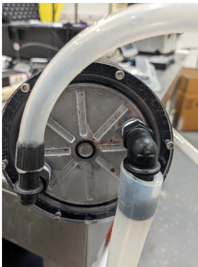
Figure 4.1.3.2-2: Krill ‘detritus’ caught in the sensor head prior to the initial through ice work (which became the medical evacuation)
