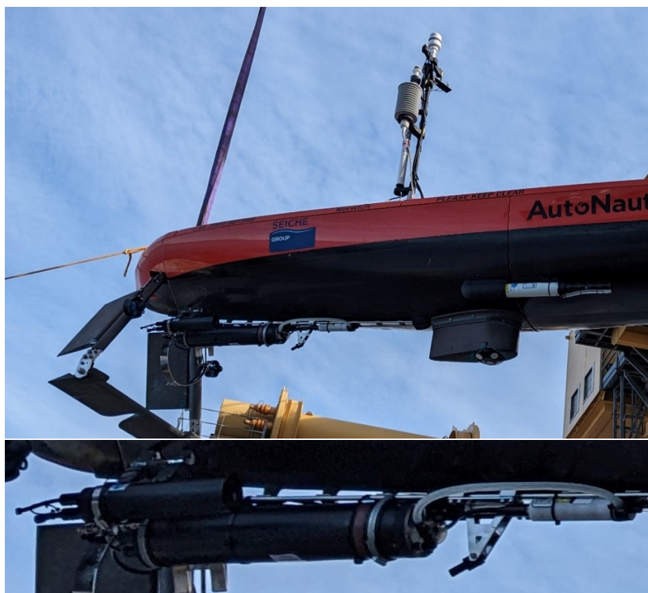
Figure 17-1: Seawater pCO 2 sensor attached to the underside of Caravela. The seawater pump is in front of the sensor (to the right in the picture), and the outlet tubing extends behind.
