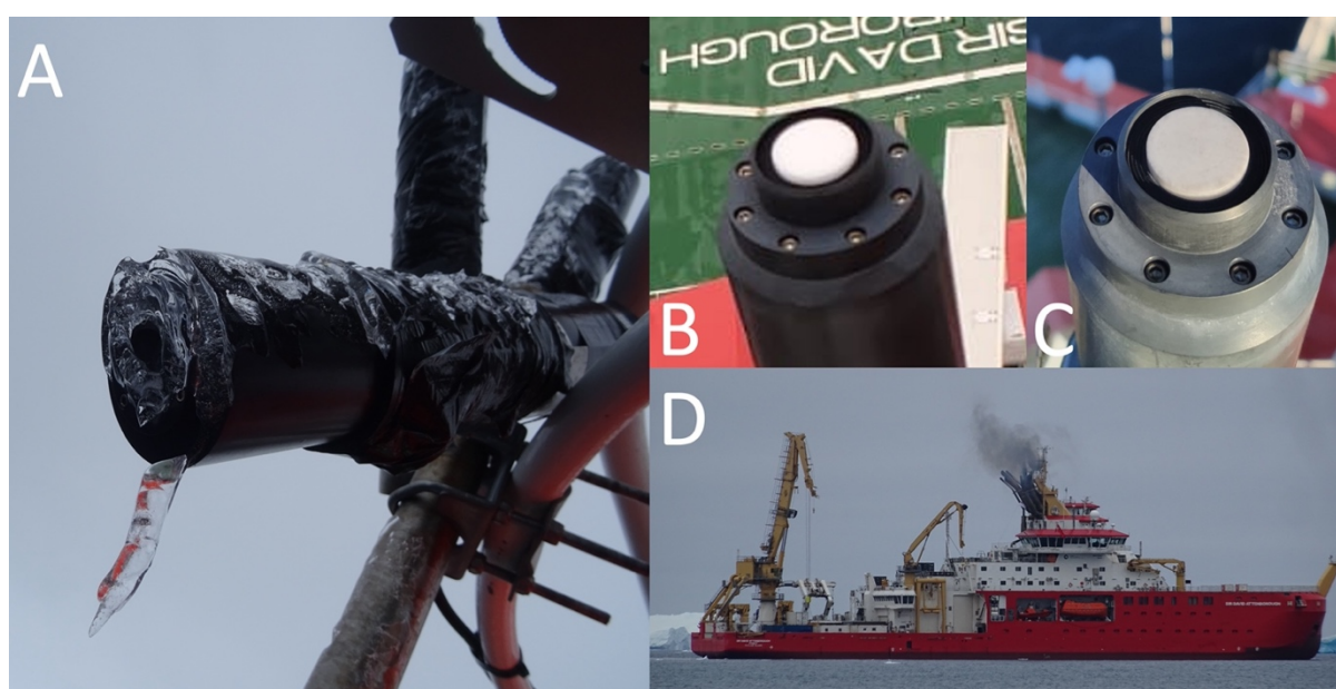
Figure 4.3.2-4: (A) Photo on the 11 th of February of ice that grew on the water-leaving radiance sensor. (B) Photo of irradiance sensor when mounted at the start of the cruise and (C) at the end of the cruise, prior to cleaning. Note the change in colour of the cosine collector caused by the sensor being close to the ships exhaust (see D for example of exhaust fumes from ship, taken on the 3 rd of March from Seymour Island).
