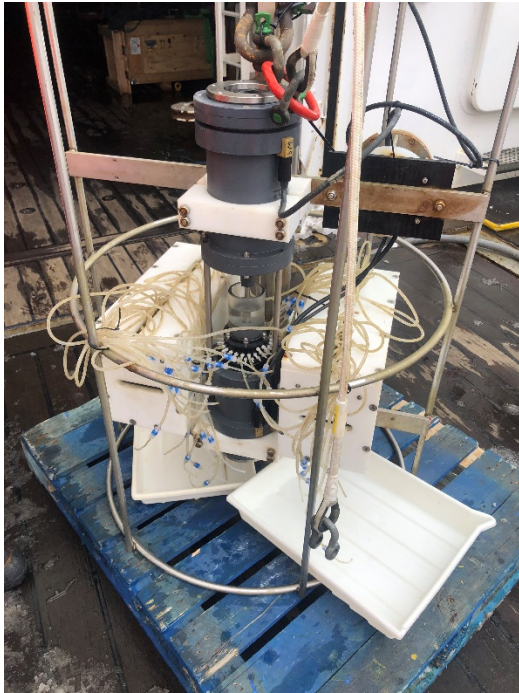
Figure 8.1-4: The AQUAMONTITOR on recovery from the long-term mooring.
