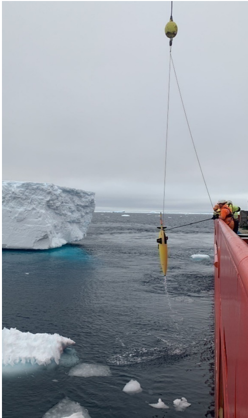
Figure 13.1-13: Seaglider lifted on board using ship's crane
