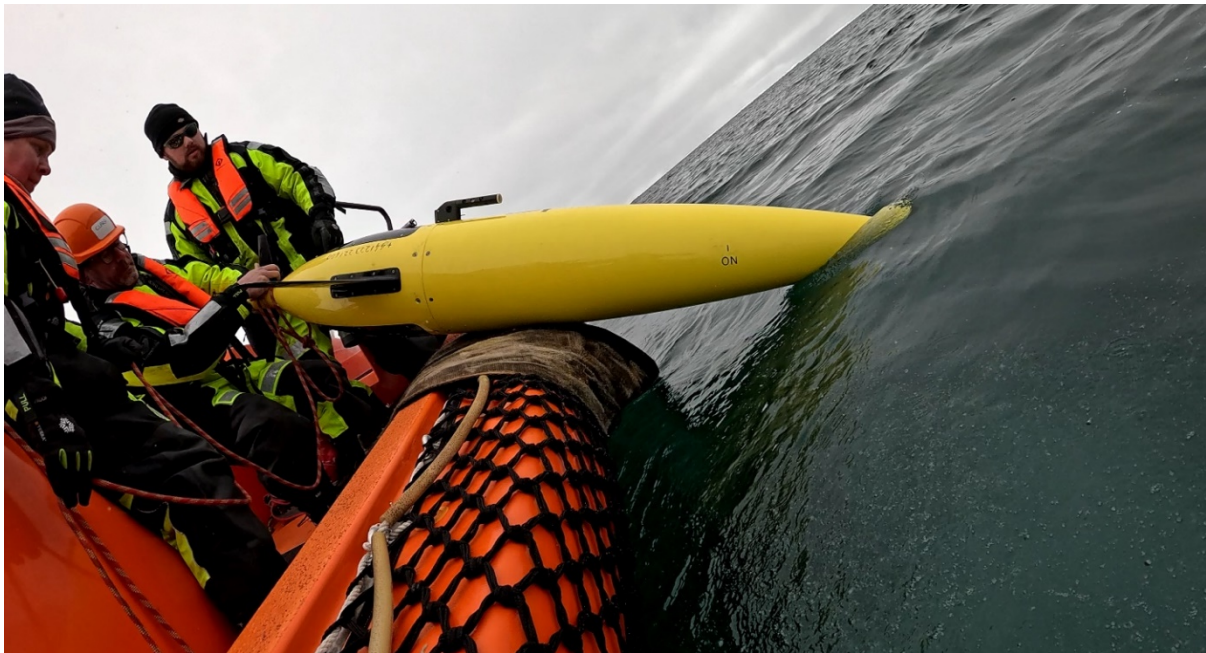
Figure 13.1-10: Deployment of Seaglider using small boat
