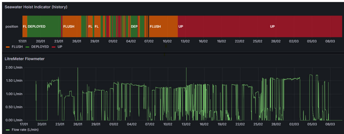
Figure 4.1-1: UCSW hoist position status (top), and UCSW sensor wall flow rate (bottom) throughout the duration of SD035 (2024-01-17 to 2024-03-09).
