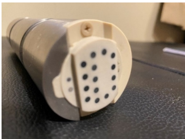
Figure 4.1.4-1: ANB electrode transducer configuration
