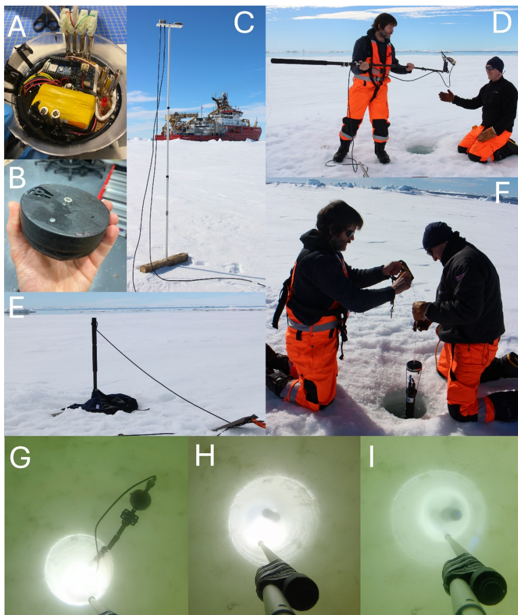
Figure 7.1.7-1. (A and B) Low-light black Sensing Secchi Disk designed to measure very low multi-spectral visible light levels. (C) Above-surface pole for collecting surface light measurements above the height of people and kit used on the ice. (D, E and G) swing arm designed to collect light measurements away from the 300 mm auger hole. (F) Profiling using the low light Sensing Secchi Disk and ECO-FLBB Backscatter and chlorophyll-a fluorescence sensor. (H and I) differences in the light environment between not covering (H) and covering (I) the auger hole, as seen from a Go-Pro.
