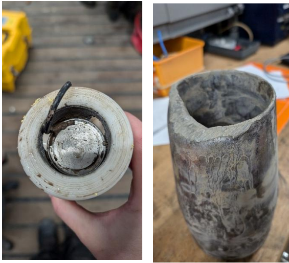
Figure 8.1-1. Photographs of damaged core cutter and O-ring in the pressure release valve.
