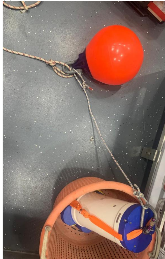
Figure 3.8-3. Drifting ADCP set up on (a) before deployment, (b) during deployment.
