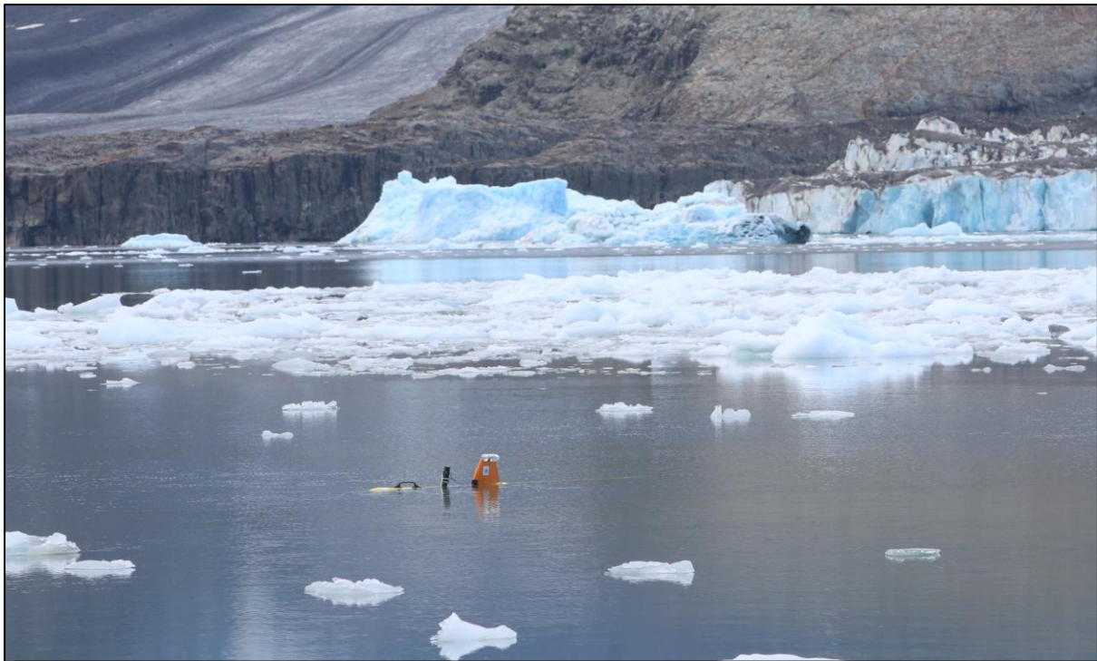
Figure 5.2-1. Freya surfaces after a failed mission near a meltwater plume and southward moving ice raft. Surface (glacial) ice coverage was hard to predict due to meltwater plume induced current close to the glacier. Photo: Lewis Drysdale.
