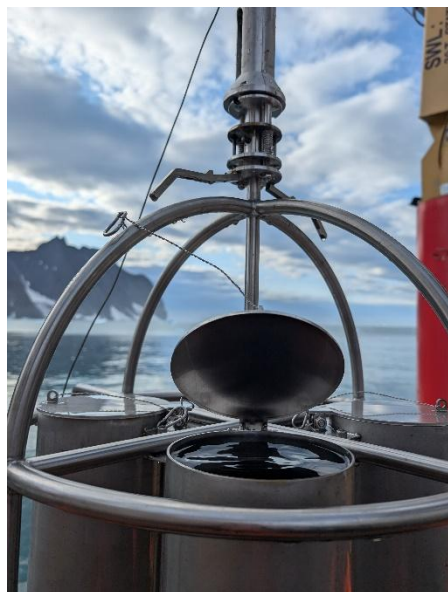
Figure 8.1-2. Photo of unclosed bottle on sediment trap.
