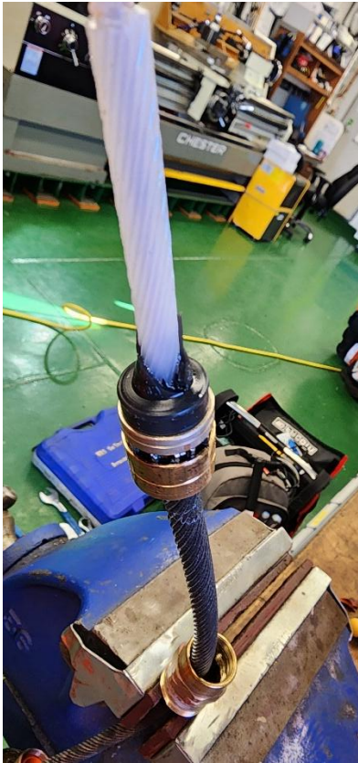
Figure 7.2-15. Broken sleeve in OFJB found after overloading.
