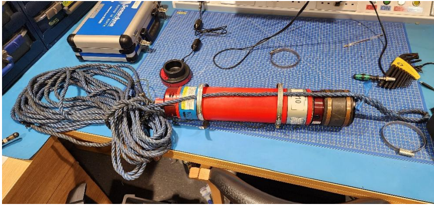
Figure 7.4-1. USBL setup for test the system on Erebus.
