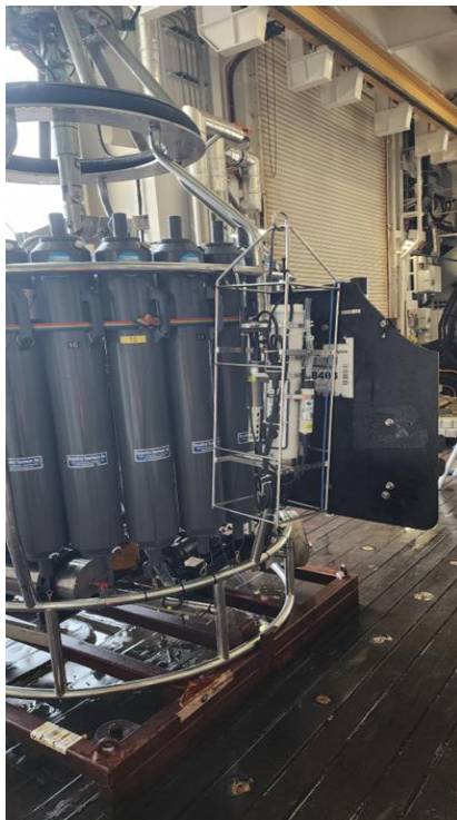
Figure 7.2-12. SB19 attached to the CTD (left), SB19 and Idronaut attached to the CTD (right).
