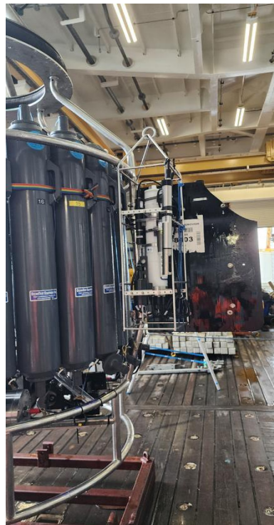
Figure 7.2-12. SB19 attached to the CTD (left), SB19 and Idronaut attached to the CTD (right).
