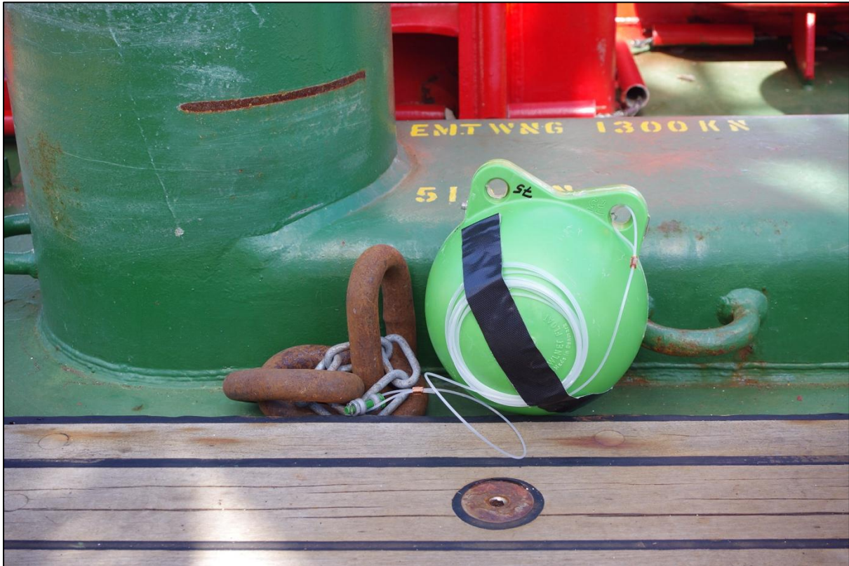
Figure 3.10-3. LoTUS buoy 75 on deck prior to deployment, with the tether still taped to the buoy.
