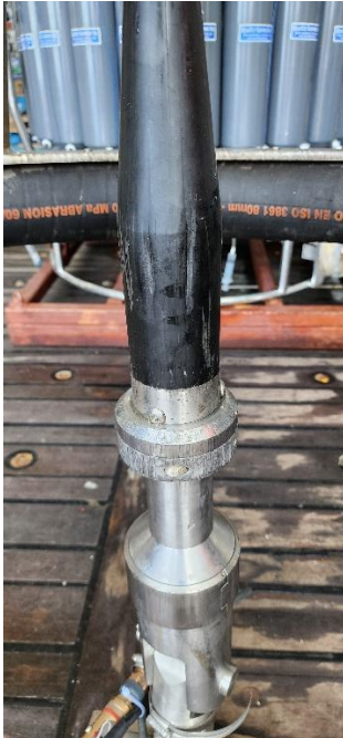
Figure 7.2-13. Bullet after overload.
