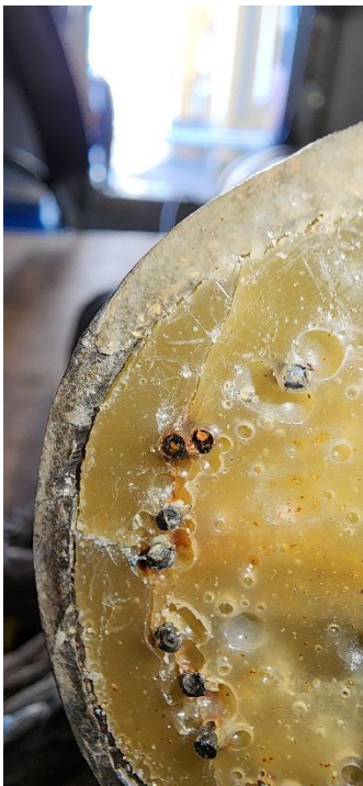
Figure 7.2-14. Cracks in mechanical potting after overload.
