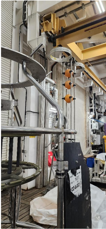
Figure 7.2-17. Pin welded back on collar.
