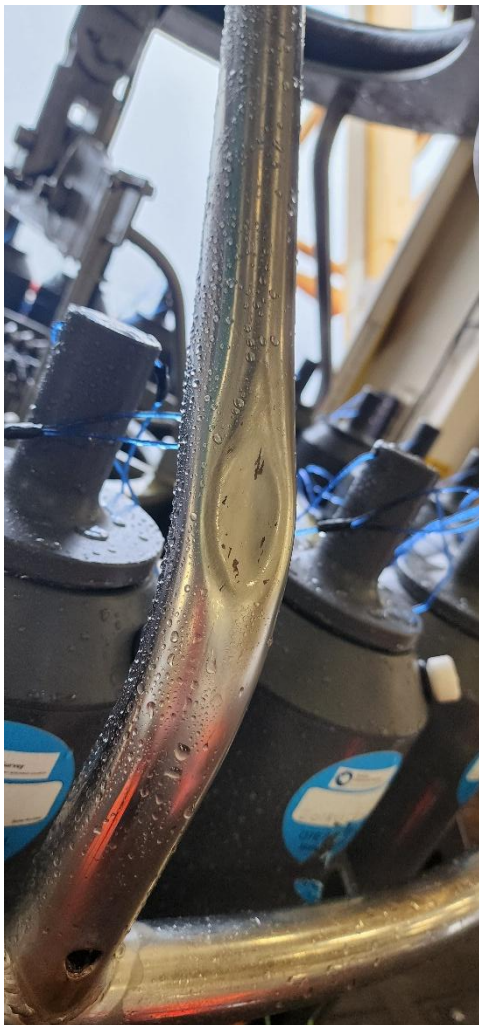
Figure 7.2-9. Piece of fin broken off during recovery.
