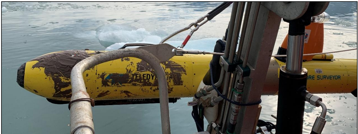
Figure 5.2-3. Freya after ROF-M6 showing signs of collision with the seabed. Photo: Lewis Drysdale.
