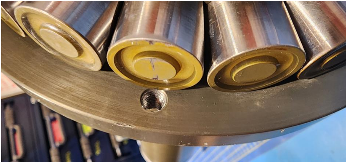
Figure 7.2-7. When the original SBE32 was removed, one of the bolts broke off. it was drilled out and re-threaded, however some damage on the solenoid can be seen.
