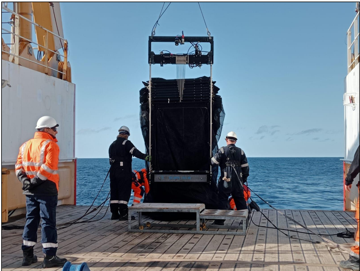
Figure 4.3-1. MOCNESS being deployed during SD041.
