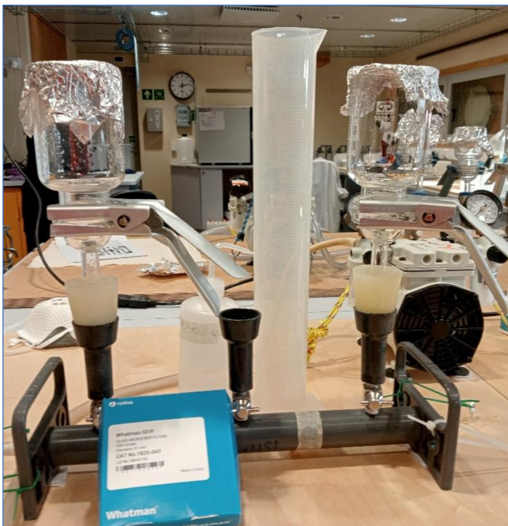
Figure 4.9-1. Filtration system for isotope analyses.
