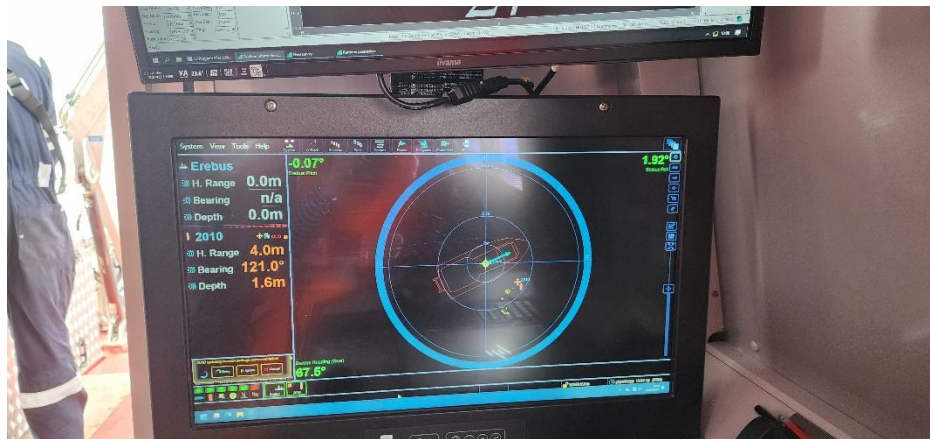
Figure 7.4-2. USBL screen showing it picked up the beacon.
