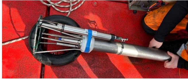
Figure 3.8-2. MSS deployment using free sinking-method and hand recovery. (a) Lea demonstrates the free sink method. (b) Lea demonstrates manual recovery. (c) Calibration set up using Idronaut CTD.
