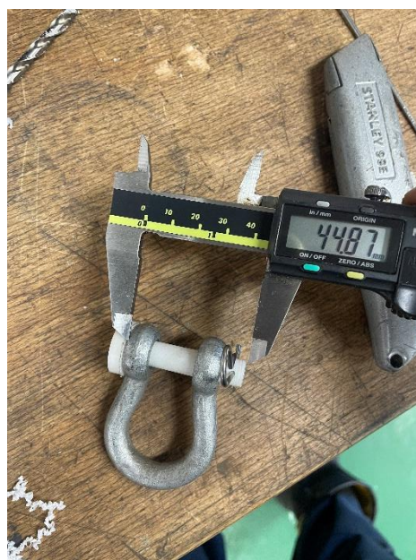
Figure 8.1-3. PTFE pin in the 2T shackle.
