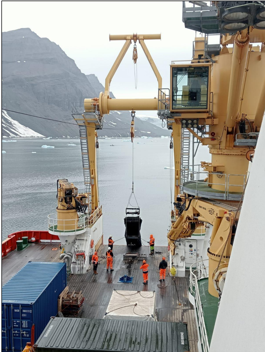
Figure 4.3-2. MOCNESS deployment showing deployment method on SD041.
