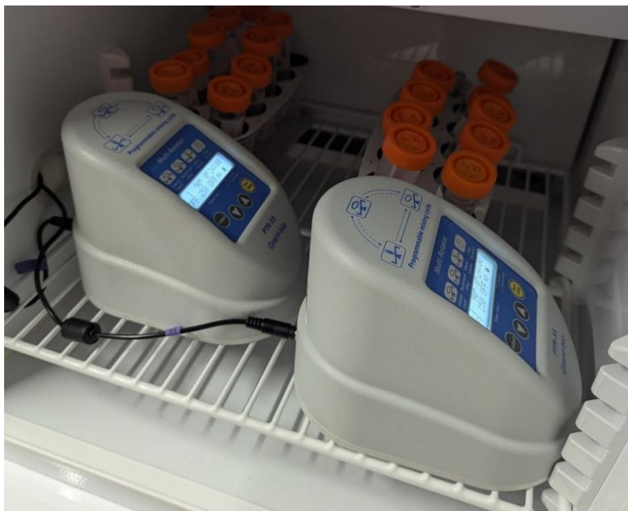
Figure 4.6-2. The experimental setup with the rotators and the Falcon tubes inside the refrigerated incubator.
