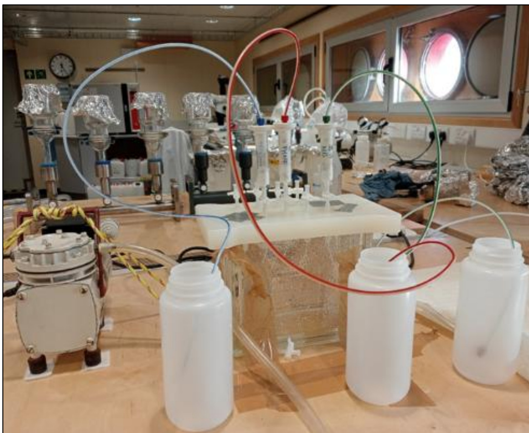
Figure 4.11-2. Solid Phase Extraction (SPE) vacuum manifold system used during SD041.
