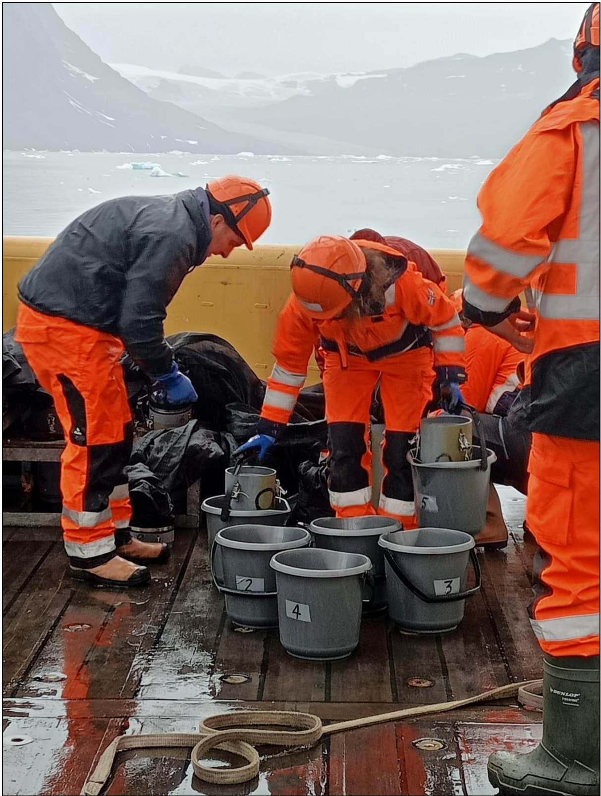
Figure 4.3-3. MOCNESS recovery during detachment of cod-ends (cod-ends resting in grey buckets here).
