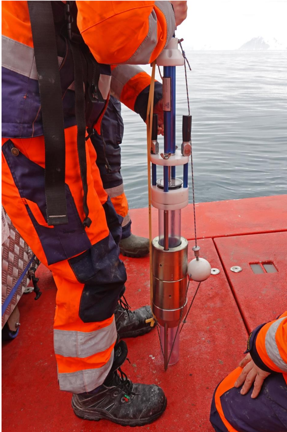
Figure 12: Gravity core set-up (photo credit J. Oliver)
