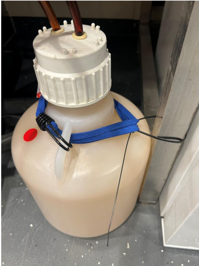
Figure 4.3: Modified assembly and securing of carboy
