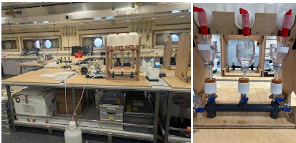
Figure 3.4: Filtration rig used on SD049
