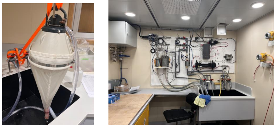
Figure 3.3: Underway sampling using mini bongo and planktoscope: onboard the SDA during SD049 to collect zooplankton samples the Main Lab for collecting zooplankton samples via a Mini Bongo net (left) and from the Uncontaminated Sea Water Laboratory for passing through a planktoscope (right).
