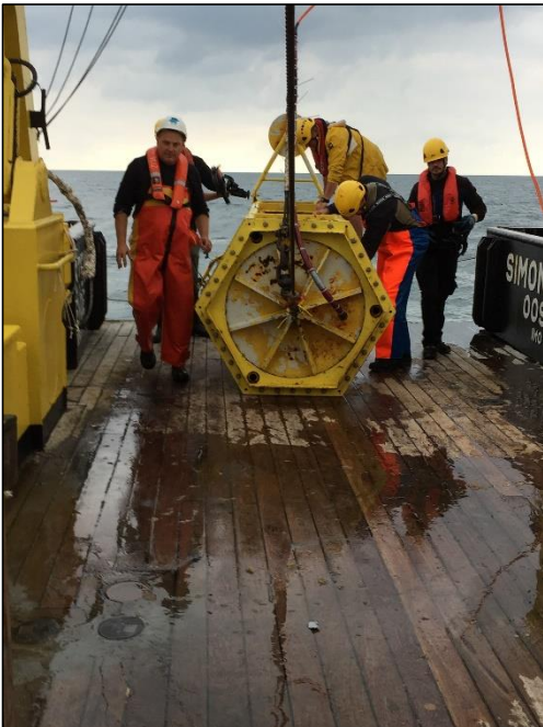
Figure 8 – Recovering the core from the vibrocore on the deck of RV Simon Stevin
