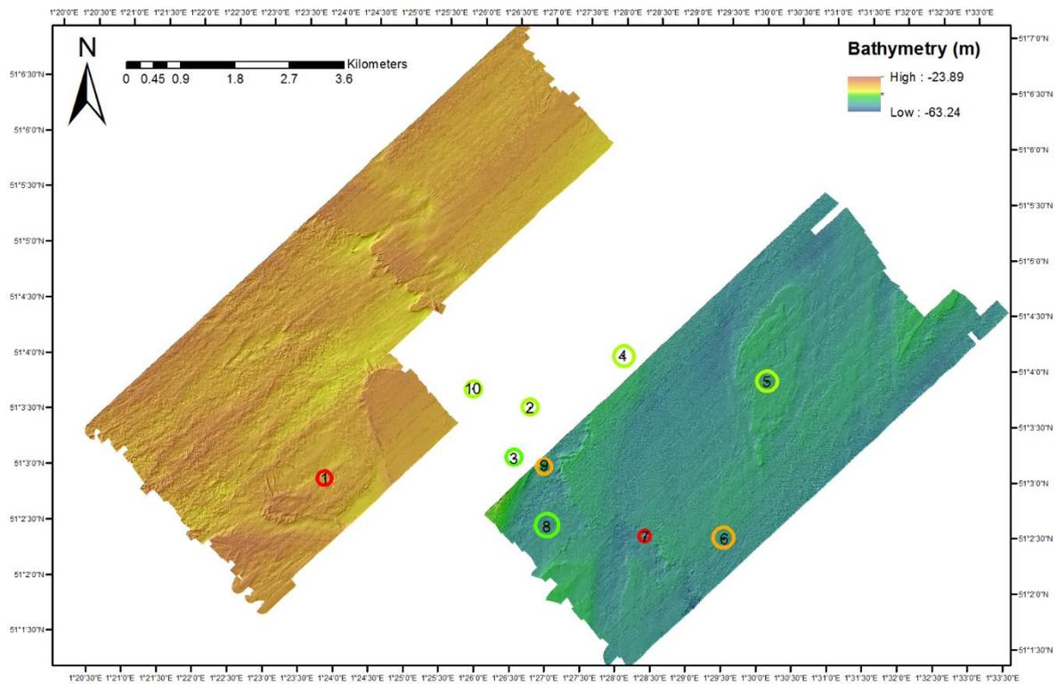
Figure 2: Preliminary bathymetric image of the 2019 survey (unprocessed data) with sample stations indicated.
