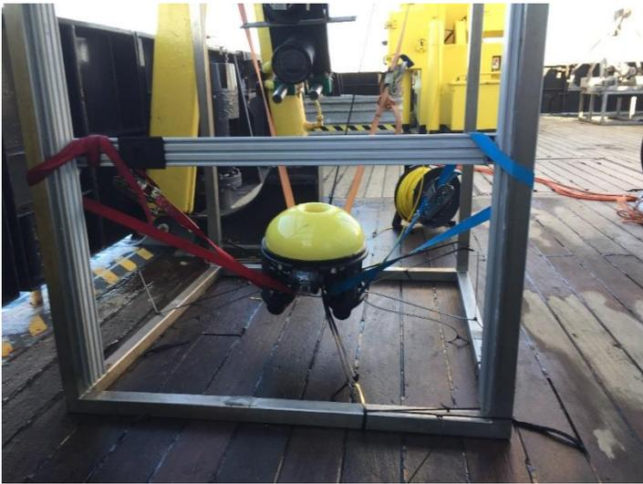
Figure 4. Mini-ROV mounted inside the VLIZ video frame.
