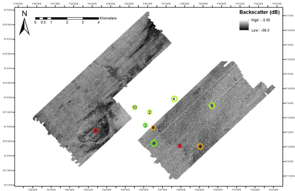
Figure 3: Preliminary backscatter image of the 2019 survey (preliminary processing to 1m resolution) with sample stations indicated.
