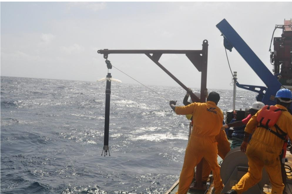
**Figure.** Vertical microstructure profiler retrieval during BOBBLE cruise.
