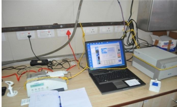
Radiosonde check and receiver setup
