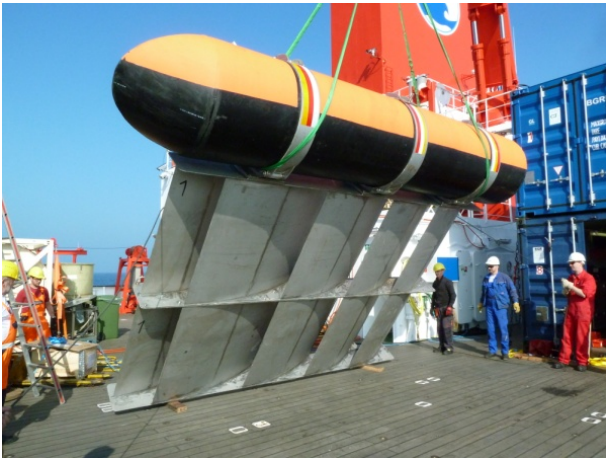
A paravan for deflection of 3D seismic equipment
