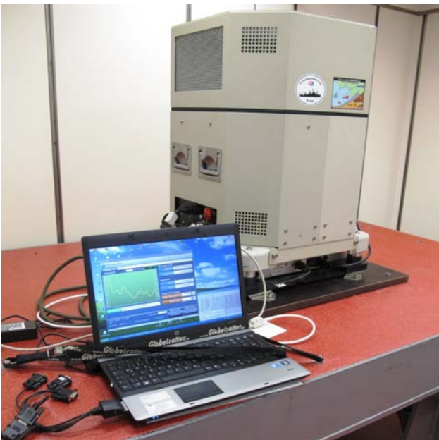
KSS32-M gravimetric sea system in the on board gravimetric room of RV SONNE
