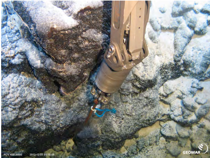
Fig. 4.4: Rock sampling in 3,500 m water depth using ROV Kiel 6000. A conventional chisel held by the manipulator of the ROV turned out to be a useful tool for rock sampling (photo: GEOMAR).
