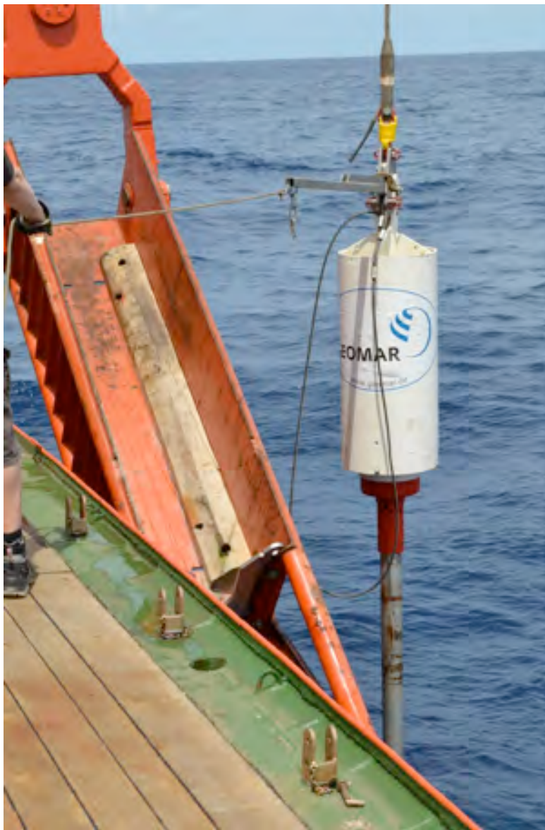
Fig. 6.14: Operation of the GEOMAR piston corer during SO-225 (right) and schematic diagram of the split-piston corer from Fa. Marinetechnik Kawohl.
