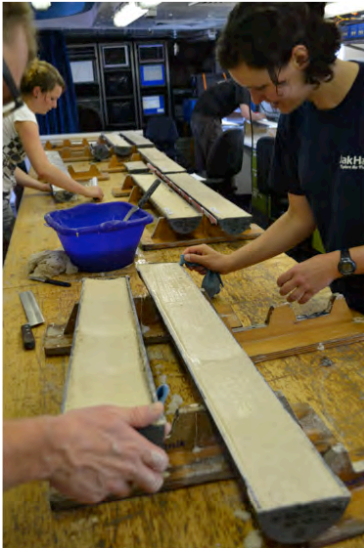
Fig. 4.6: Cutting sediment cores during SO-225. The light sediments consisting primarily of calcitic microfossils, are cut into cm-slices (photo: GEOMAR).
