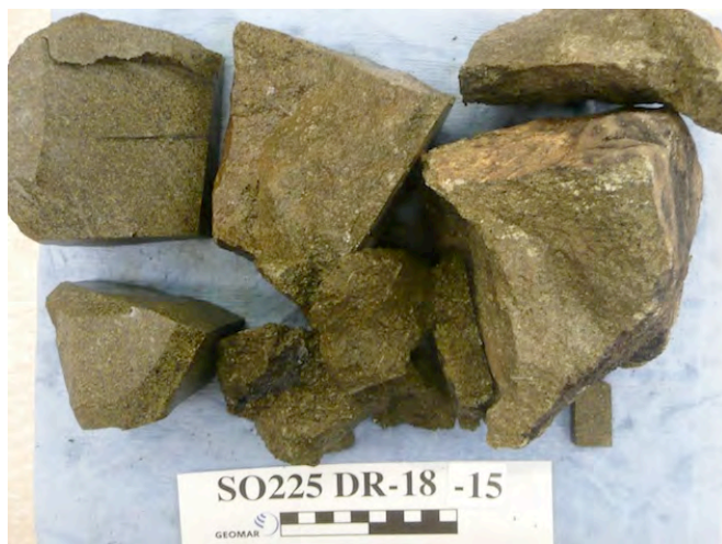
Fig. 5.31: Coarse grained greenschist with up to 1 cm long chlorite crystals.
