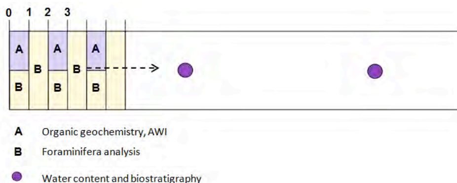
Fig. 6.16: Sampling scheme applied for SO225 sediment cores. The displayed sampling pattern is repeated every 2 cm: 0-1 cm org. geochemistry (AWI) / foraminifera geochemistry (GEOMAR/AWI), 1-2 cm foraminiferal (GEOMAR/AWI).
