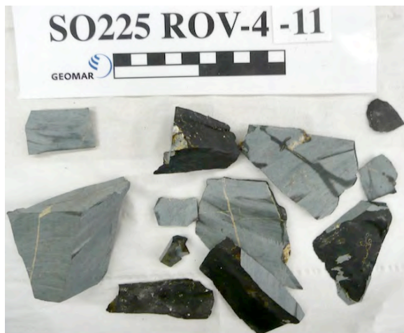
Fig. 5.21: Fairly fresh aphyric lava sample with abundant filled veins / cracks.
