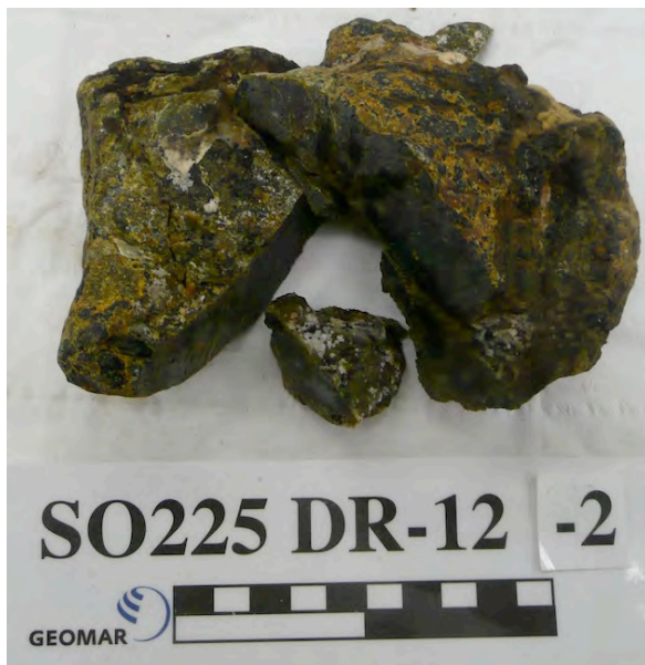
Fig. 5.27: Large volcanic glass fragment with green palagonite on the outside and fresh black glass in the interior.
