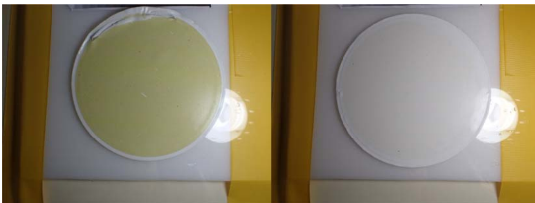
Figure 7.16 Examples for filters from station SO245-08. Left: 200 m water depth (=DCM, pumped volume: 1317 liters), right: 2800 m water depth (pumped volume: 1158 liters).
