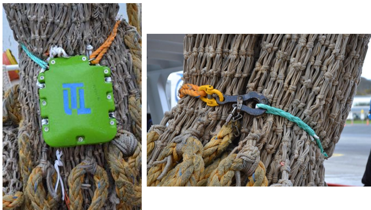
Figure 13: FossTech's prototype Catch Limitation Release (CLR). Left: CLR unit fitted to codend. Right: restrictor line and fastenings.
