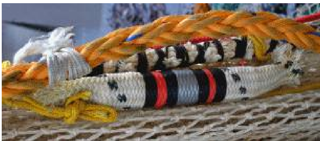
Figure 9.2 – a depth sensor (SXL-0154) in its protective housing and sheath fixed to the top of the FRS.
