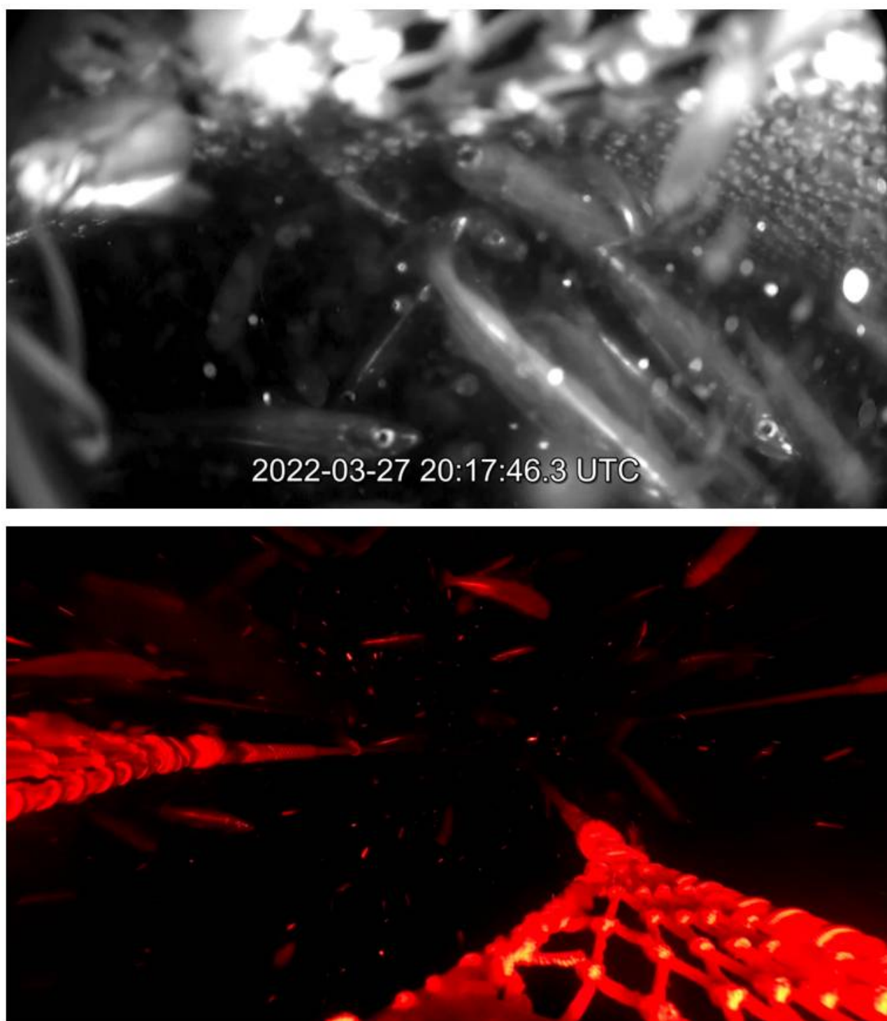
Figure 3.5 – Images from video taken during haul 03 at 20:17, 16 minutes before the start of haul-back at 20:33. Top: from position 5iB looking aft toward the fish-lock and cod-end, showing high densities of fish in the top of the FRS. Bottom: from position 2iF, looking forward over the escape opening, with medium densities of fish passing over the escaping open. Note – the escape rate was approximately 65 fish/minute [20:17 - 20:18].
