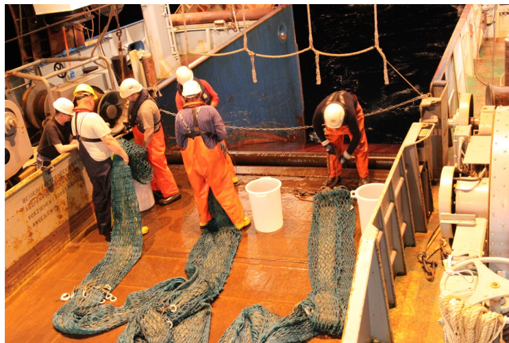
Fig. 2. Cod-ends of the pelagic multi-sampler used with the large trawl (Photo: K. Wysujack)
