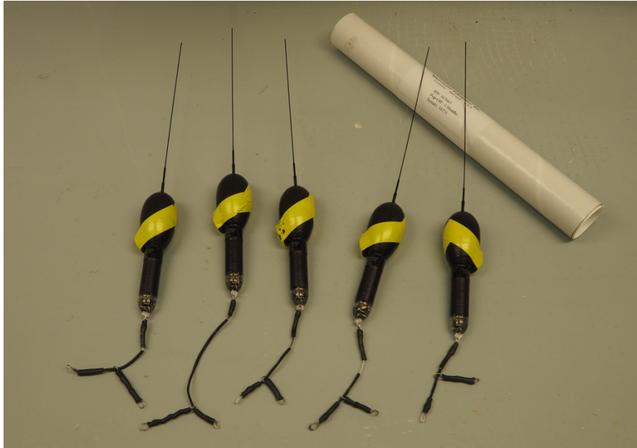
Figure 5. The satellite tags measure 120 mm in length (without antenna) and weigh 40g. (© Lasse Marohn)
