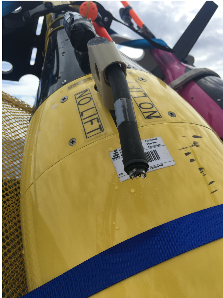
Figure 6: The damaged CT sensor on SG534.
