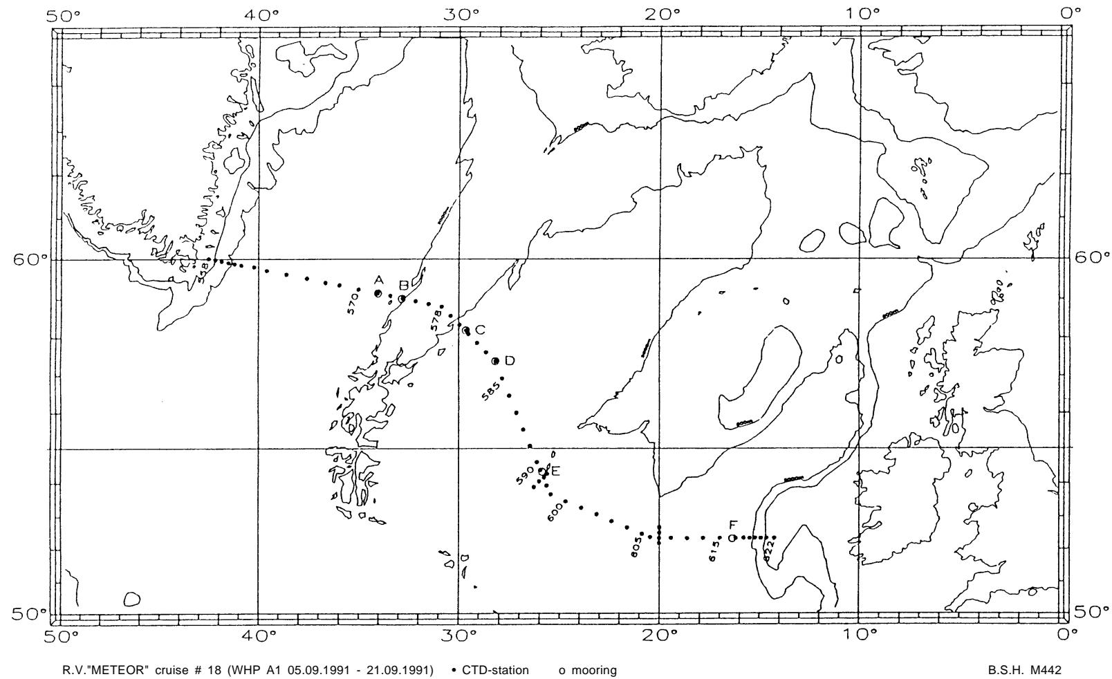
Figure 1: The WOCE A1-cast section. CTD02-stations are marked by dots. Station numbers are indicated. The circles denoted A to F are locations of moored current meter arrays.
