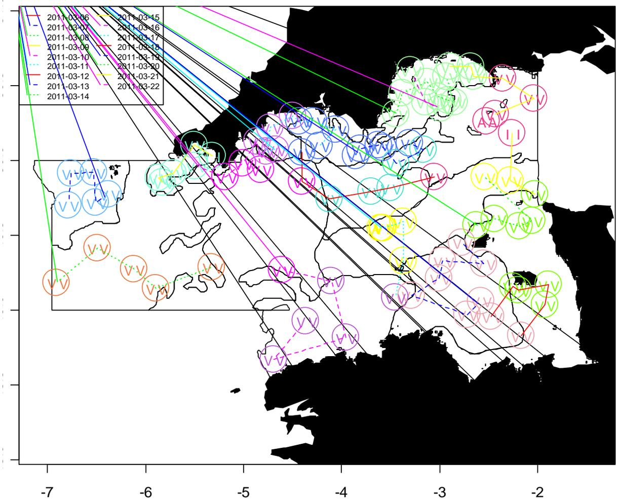
**Figure 2:** Survey Track showing beam trawl stations and validity codes by day
